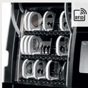
Integrated and RFID-controlled blank tank
