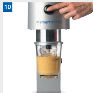
10 Smartmix mixes the dental arch plaster
