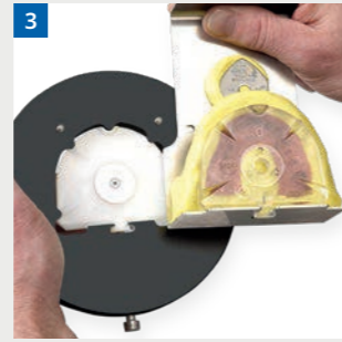
3 With the Giroform base plate inserted, the impression carrier is attached to the plate holder
