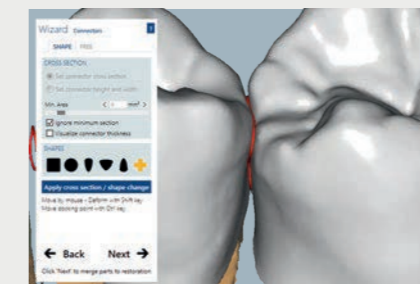
Connect contact surfaces with each other for more aesthetic interdental spaces
