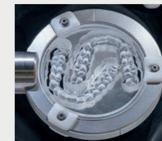
Easy, reproducible splint fabrication using Ceramill CAD/CAM
