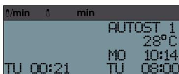
9. The finishing time as well as the calculated switch-on time are shown in the display.
