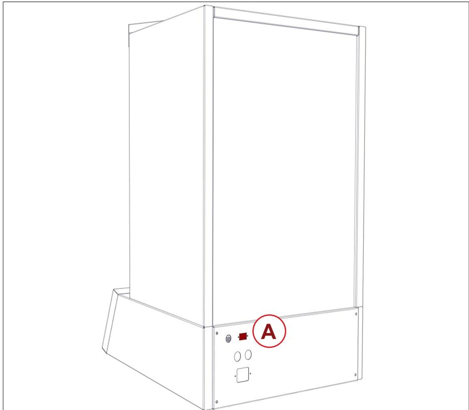
The sintering oven has an RS-232 interface (A) on the rear, which is used to save log files on a computer.
